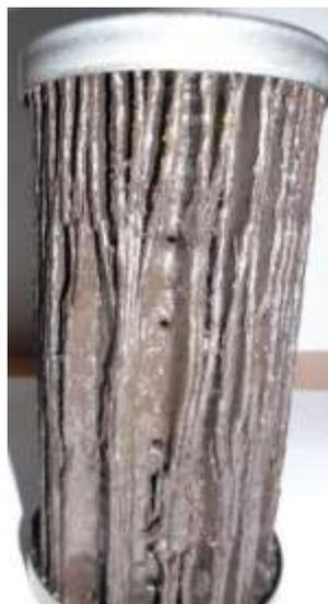
On another system I worked on there was no indicator on the return filter and valves were failing. We removed the element and found it had partially collapsed, because it had not been changed. The filter was made of cellulose and it had a 30 micron Beta Ratio of 200. Not good
